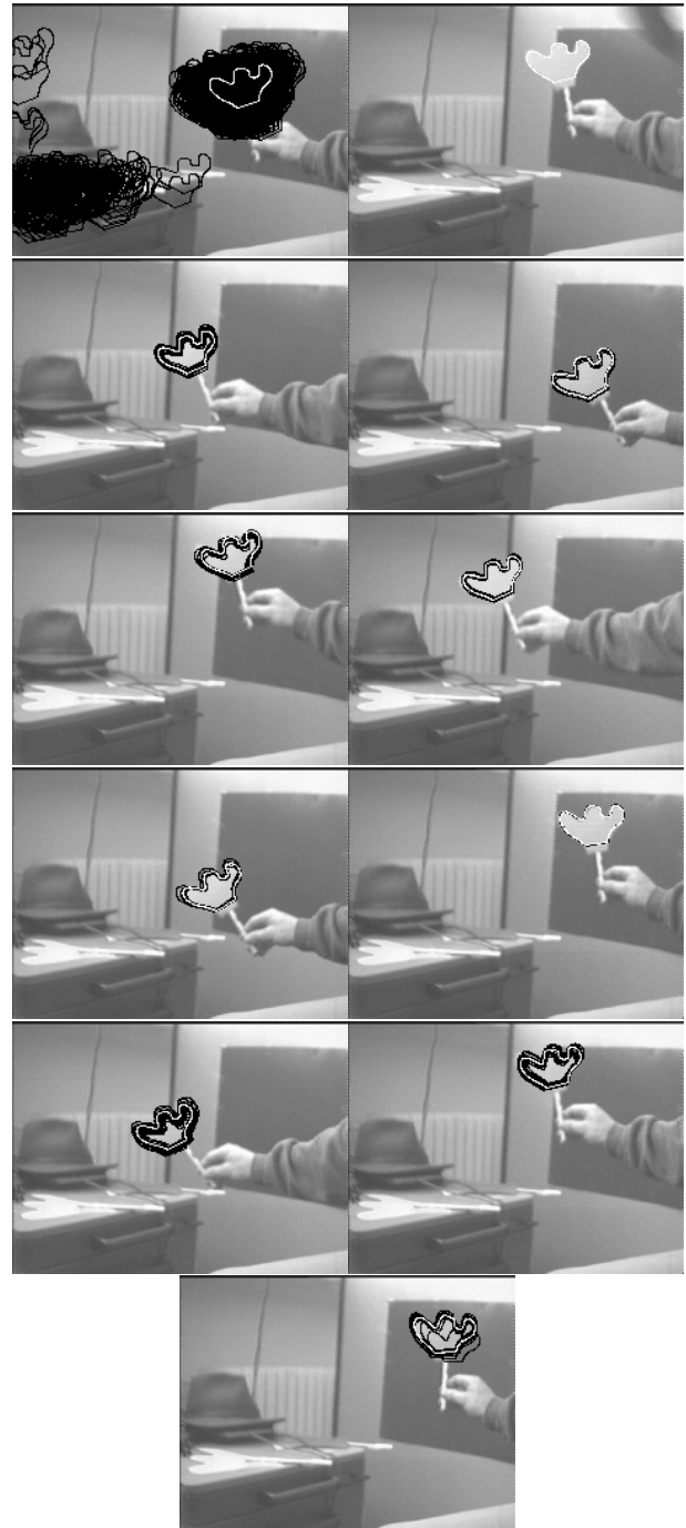
Figure 5: A typical tracking sequence with RB-SS-HS-SIR and 600-particles. Black contours show configurations with high probabilities, while the white contour represents the expected configuration. Note that there is an object lying on the table that has the same characteristics (e.g. is made of the same material of the same color) as the object to be tracked, making the tracking task more difficult.
