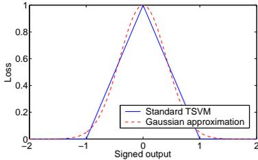
Figure 2: TSVM cost functions for unlabeled data.
