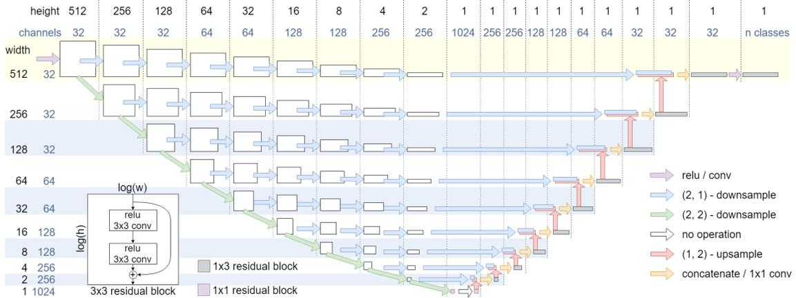
Figure 1: Proposed network architecture for 2D images to 1D segmentation. The white squares represent the size (log-scale) of the feature maps. Within each square, two convolutions are applied in a residual manner. For visualization purposes, the feature maps with width/height 1, have the same size as the feature maps with size 2. In the upsampling path, the residual blocks have height 1, and the convolutional kernels are of size  $1 \times 3$ .
