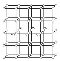
Figure 7: MRF model (a M×N×2 grid graph) for optical flow problem.
