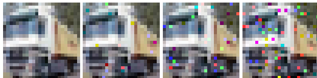
Figure 1. An example of clean and contaminated images. We apply the salt and pepper noise to each pixel. The probabilities of noisy pixels are 0%, 1%, 2%, and 4% from left to right, respectively.
