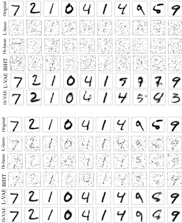
Figure 1. Examples of reconstructed images with 50 measurements (top) and reconstruction with 200 measurements (bottom) on the MNIST dataset.
