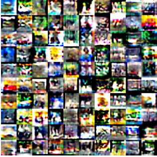
Figure 8. Samples generated by GTN to teach CIFAR10 are unrecognizable, despite being effective for training. Each column contains a different class, and each row is taken from the same inner-loop iteration (evenly spaced from all 128 iterations, early iterations at the top).
