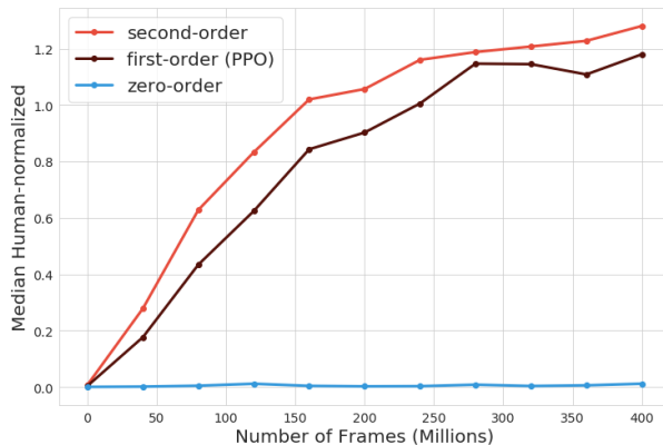
Figure 6. Near on-policy optimization. The x-axis is the number of frames (millions) and y-axis shows the median human-normalized scores averaged across 57 Atari levels. The plot shows the mean curve averaged across 3 random seeds. We observe that second-order expansions allow for faster learning and better asymptotic performance given the fixed budget on actor steps.
