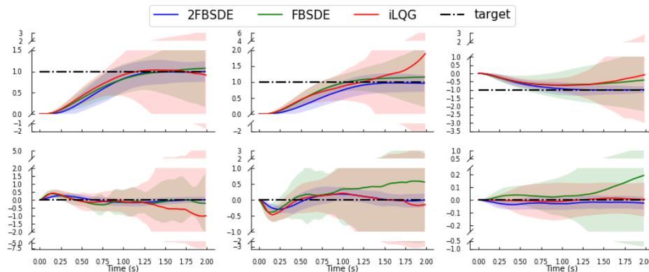
Figure 4: Above plots, from left to right, in the top row are  $x$ ,  $y$  and  $z$  positions and bottom row are roll, pitch and yaw angles. 2FBSDE clearly out-performs both FBSDE and iLQG, as indicated by the smaller variance in all states and stability while others diverge due to high noise.
