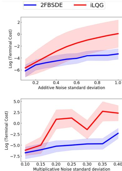
Figure 5: **Human Arm Planar Reaching Task:** 2FBSDE has lower mean and variance of terminal cost compared to iLQG.
