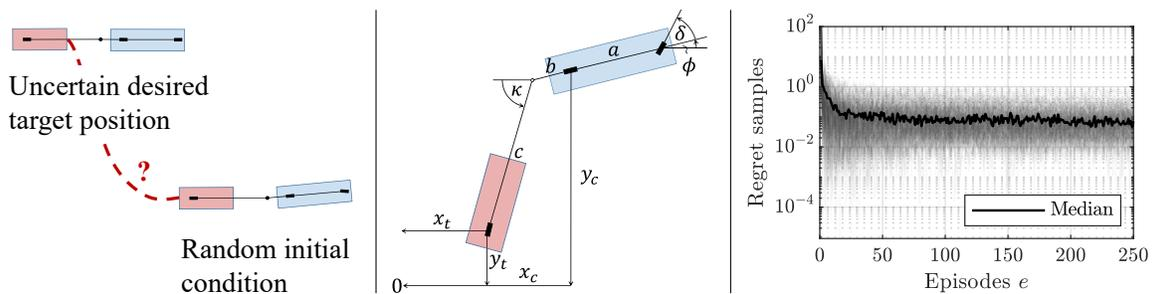
Figure 1: **Left:** Problem setting of steering a partially known trailer system from a random initial condition to an uncertain target position. **Middle:** Car-trailer system. **Right:** Sampled regret  $\Delta_e$  and median of 200 different systems over 250 learning episodes.
