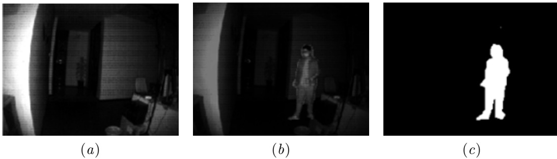
Figure 5: The input and label of the algorithm for training are shown here. (a) Intensity map acts as background for the input. (b) Intensity map acts as contrast for the input. (c) Foreground (Actual Difference) acts as label for output.
