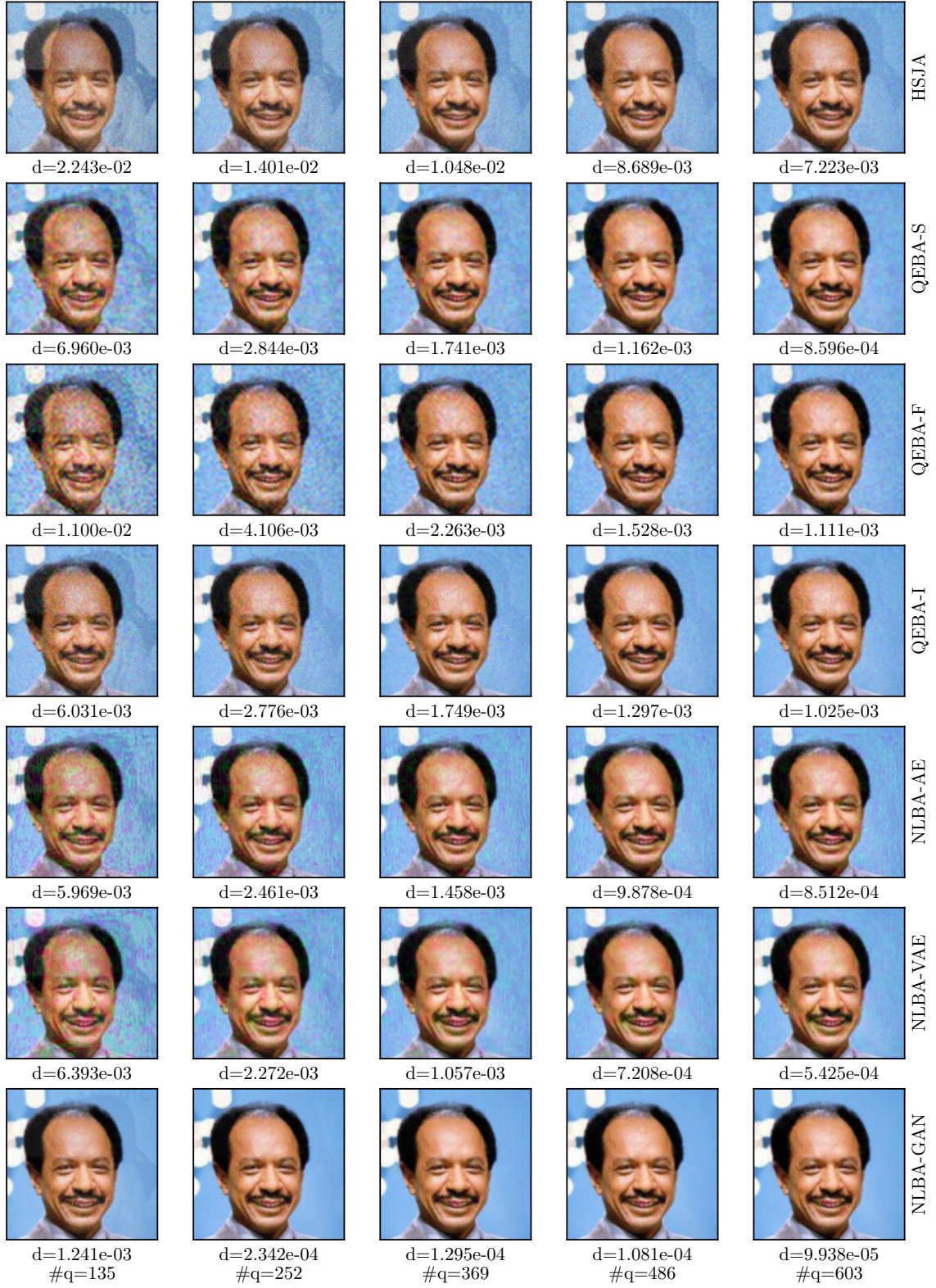
Figure 11: The attack performance of all the NonLinear-BA methods and the baseline methods on one pair of image of the CelebA dataset. The source-image and target-image of this case study are shown in Figure 4. The d in the figure denotes the perturbation magnitude (mean squared error) of the adversarial example with respect to the target-image. The \#q values are the number of queries used at the point for each column.
