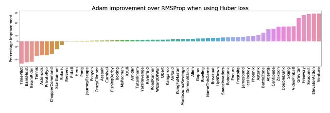
Figure 14. Comparing Adam vs RMSProp when both optimizers use the Huber loss.
