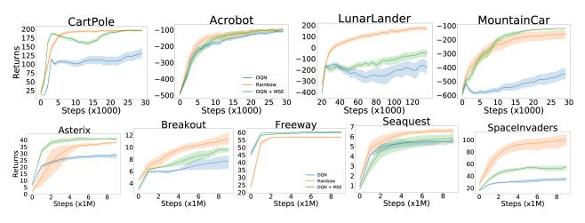
Figure 13. Evaluation of the use of the mean-squared error loss, instead of the Huber loss, in DQN.
