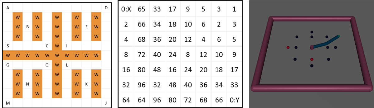
(a) GridWorld with start (S), walls (W), goal (G), objects (other letters), (b) Terrainworld with numbers indicating terrain types (c) Reacher with red active and black inactive targets
