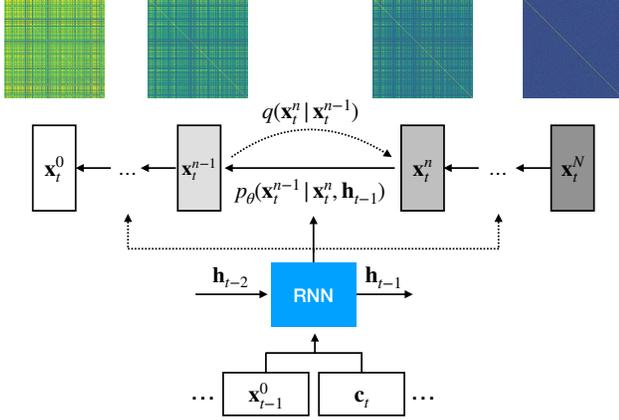
Figure 1. TimeGrad schematic: an RNN conditioned diffusion probabilistic model at some time  $t - 1$  depicting the fixed forward process that adds Gaussian noise to the signal and the learned reverse processes. The cross-correlation of the time series is also depicted during the stages of the process, from white noise (right) to the original signal (left).
