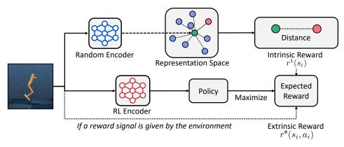
*Figure 2.* Illustration of our approach. The intrinsic reward for each observation is computed as the distance to its *k*-nearest neighbor, measured between low-dimensional representations obtained from the fixed random encoder. The intrinsic reward is then combined with extrinsic reward from the environment, if present. A separate RL encoder is introduced for a policy that maximizes expected reward.
