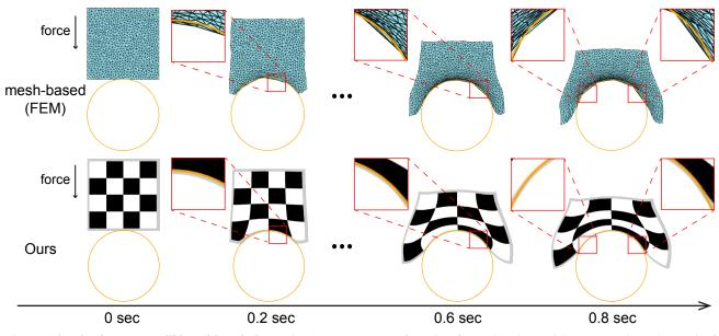
*Figure 7.* **An elastic square collides with a circle.** Under the same memory footprint (for storing the spatial representation), the result of mesh-based FEM (top) conforms poorly at the collision interface. In contrast, our result (bottom) fits the boundary more gracefully.
