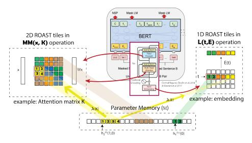
Figure 1. Generic model compression with operation-specific blocking for BERT as an example: (left) Shows how 2D tiles are mapped to  $\mathcal{M}$  in case of  $\mathbf{M}\mathbf{M}$  operation. (right) Shows how 1D tiles are mapped to  $\mathcal{M}$  in case of  $\mathbf{L}$  operation.  $\lambda$  is the module-specific GMS scaling factor
