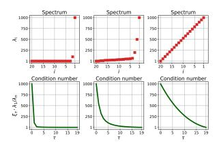
Figure 3: *Above:* different distributions of eigenvalues  $\lambda(B)$ . *Below:* the corresponding improvement of the condition number  $\frac{\beta}{\alpha} = \xi_{\tau}(\lambda) \cdot \lambda_1 / \lambda_n$  by using the preconditioner  $P_{\tau}$  of order  $\tau$ .
