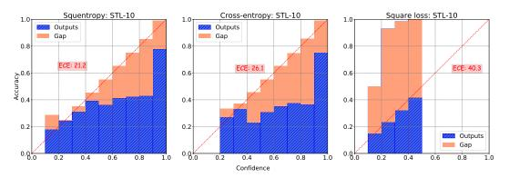
Figure 15. Reliability diagrams for a Resnet18 on STL10. Left: squentropy, middle: cross-entropy, right: square loss.
