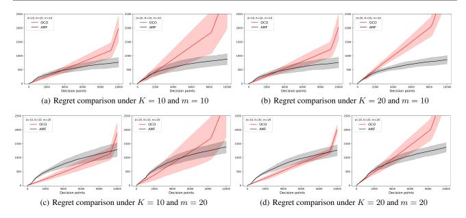
Figure 5. Regret comparison of AMF and OCO algorithms under  $B = \sqrt{dT}$ . The line and shade represent the average and standard deviation based on 20 repeated experiments.
