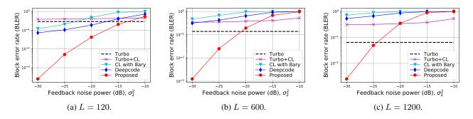
Figure 11. BLER of various selections of blocklength L with r = 1/3 when the forward SNR is -1dB.
