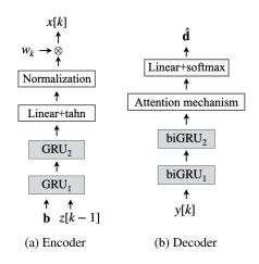
Figure 8. Encoder and decoder in a compact structure.
