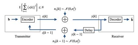
Figure 1. A point-to-point AWGN communication channel with noisy feedback.
