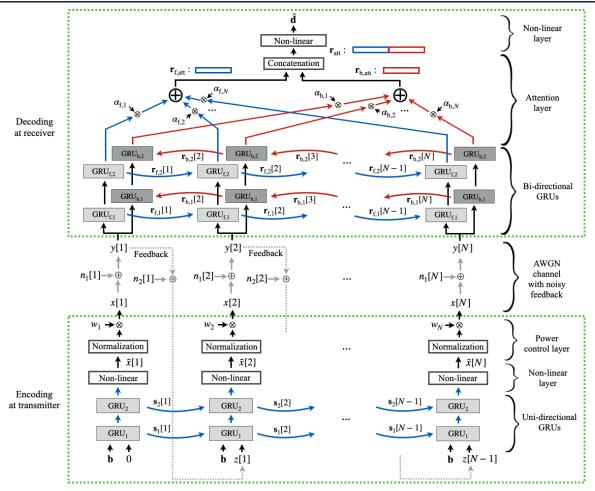
*Figure 2.* Our proposed RNN autoencoder-based architecture for non-linear coding over an AWGN channel with noisy feedback. At the end of the decoding process,  $\hat{\mathbf{d}}$  denotes the probability distribution of  $2^{K}$  possible outcomes of the bit stream estimate  $\hat{\mathbf{b}}$ . A compact form of the architecture is included in Appendix C.
