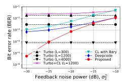
Figure 4. BER with medium/long blocklength L and rate r = 1/3 when the forward SNR is low (-1dB). Our feedback codes significantly improve BER performances compared to other feedback schemes over a wide range of feedback noise powers.
