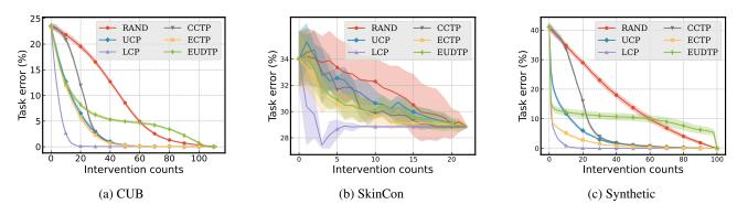
Figure 3: Intervention effectiveness of concept selection criteria (task error vs. number of concepts corrected by intervention) measured on I+S level. A more effective method would reduce the error more for the same number of concepts intervened.
