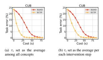
Figure 13: Comparison between concept selection criteria in terms of the intervention cost for the CUB. Here, cost represents the seconds for concept annotation time and inference times for g, f.
