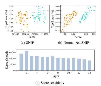
*Figure 3.* (a) The SNIP scores are uncorrelated with the test accuracy of various subnets in two isomers. (b) The SNIP scores with the layer normalization have significant positively correlation with the test accuracy of various subnets in the two isomers. (c) The growth of the SNIP score in each layer with the increase of the MLP ratio from 3.5 to 4.
