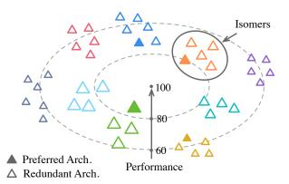
*Figure 1.* PreNAS first identifies the preferred architectures via zero-cost proxies within similar architectures, denoted as isomers, and then performs concentrated one-shot learning on only preferred architectures to achieve better convergence. The size of triangles implies different resource consumption of the architectures.
