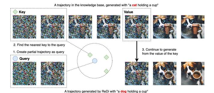
Figure 2. The inference procedure of REDI. The upper part is a complete trajectory generated by Stable Diffusion to build the knowledge base. The lower part is a trajectory generated by REDI with some intermediate steps skipped.
