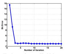
Figure 2. The objective function of Eq.(1) decreases as iterations of our block coordinate descent continue. 'Bit Error' refers to the number of bits that differ in the obtained binary codes from two different views. (32bit code learning)
