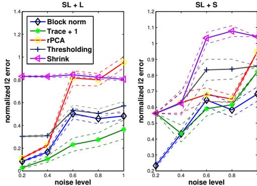
Figure 2. Comparison of the performance of various algorithms on decomposing a signal onto sparse-low rank and other component.
