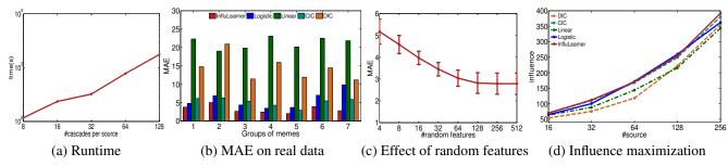
*Figure 2.* (a) Runtime in log-log scale; (b) MAE on seven sets of real cascade data; (c) The performance gain of using different number of random features; (d) Maximized expected influence of different selected sources on the real hold-out testing data.
