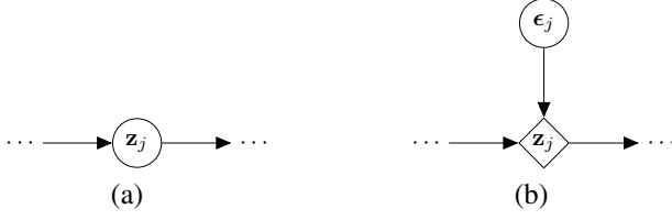
Figure 1. (a) The centered parameterization (CP) of a latent variable z_j . (b) The differentiable non-centered parameterization (DNCP) where we have introduced an auxiliary 'noise' variable \epsilon_j \sim p_\theta(\epsilon_j) such that z_j becomes deterministic: z_j = g_j(\mathbf{pa}_j, \epsilon_j, \theta) . This deterministic variable has an interpretation of a hidden layer in a neural network, which can be differentiated efficiently using the backpropagation algorithm.
