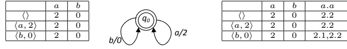
Figure 3: The initial observation table (left); corresponding one state conjecture NFM (middle); table after adding the first counterexample (right).
