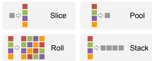
Figure 1. The four operations that constitute our proposed framework for building rotation equivariant neural networks.
