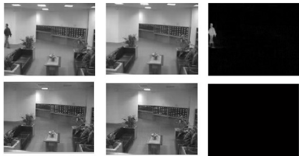
Figure 7. Two frames of a video taken in a lobby. The first column displays the original frames. The second and third columns display the LR and sparse components recovered using the proposed approach.
