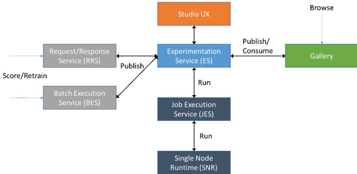
Figure 2: Component services of AzureML
