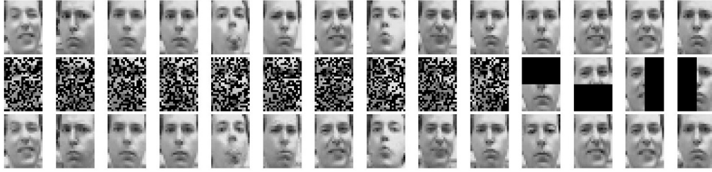
Figure 5: The first row shows the original images, second row shows the images with pixels missing, and the third row shows the reconstructed images.
