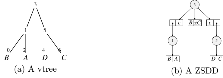
Figure 2: (a) An example of a vtree, (b) ZSDD representing the family of sets \{\{A, B\}, \{B\}, \{B, C\}, \{C, D\}\} given the vtree in (a).
