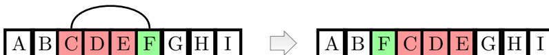
Figure 2: Example of insertion(6, 3) : the variable F is inserted in the position occupied by variable C in the initial ordering.
