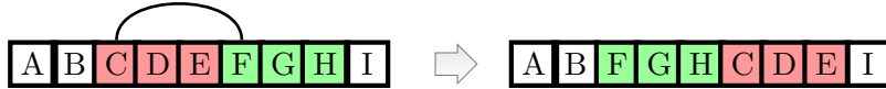
Figure 4: Example of window(6, 3, 3) : the variable F,G,H are inserted in the position previously occupied by C,D,E.
