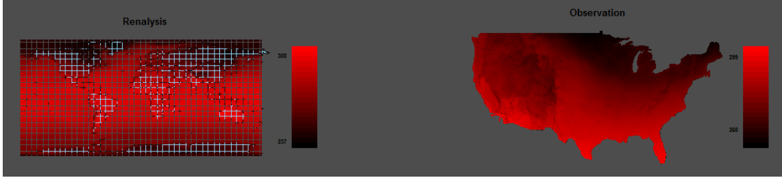
Figure 7: Example of the statistical downscaling task. Left: the climate variable (monthly mean temperature in Kelvin) with a coarse resolution at a single time point (Jan. 2009). Right: the target climate variable with a relatively finer resolution. The goal of statistical downscaling is to learn the target climate variable in finer resolution based on the historical data of the fine and coarse resolution climate data (red is larger and black is smaller).
