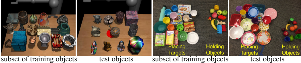
Figure 5: Training and test objects used in our simulated pushing (left) and real-world placing (right) experiments. Note that we only show a subset of the \sim 100 training objects used for the pushing and placing experiments, and a subset of the textures and object scales used for training and testing robot pushing.
