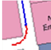
Figure 2: The LPE intention represented as a 224 \times 224 image. It captures information on the path that the robot has recently traversed (in red), the path ahead (in blue), the robot’s current position (where the red and the blue paths meet), and the local geometric environment according to the map.
