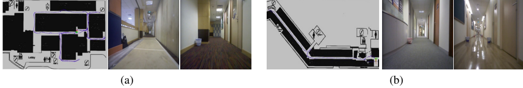
Figure 7: Generalization to a new environment. (a) The first floor of the building in robot experiments. The robot is trained on data from the first floor only. (b) The second floor, used for testing the robot, has a significantly different geometric arrangement and visual appearance.
