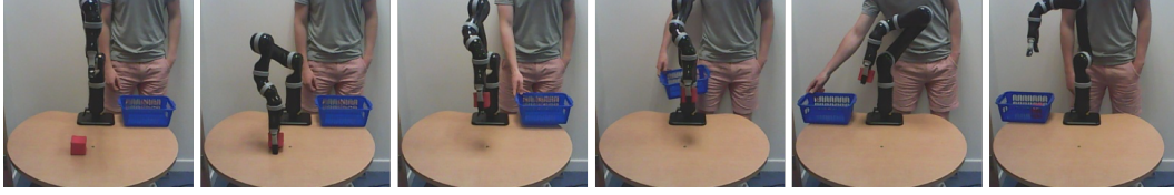
Figure 5: A sequence of images showing the network’s ability to generalise. Whilst a person is standing in the view of the camera, the robot is able to grasp the cube and proceed to the basket. As the arm progresses towards the basket, the person moves the basket to the other side of the arm. Despite this disruption, the network alters its course and proceeds to the new location. During training, the network had never seen humans, moving baskets, or this particular table.
