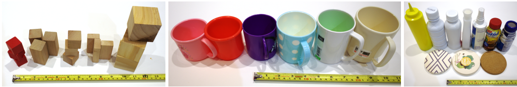
Figure 6: Left. Blocks test set. 10/15 blocks were randomly selected for each round. Center. Mugs test set. 5/6 mugs were randomly selected for each round. Right. Bottles test set. 3/7 bottles were randomly selected for each round. All 3 coasters were present in each round.
