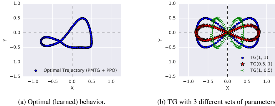
Figure 2: 2D Synthetic Control problem with a desired pattern and the TG that generates figure-eights.
