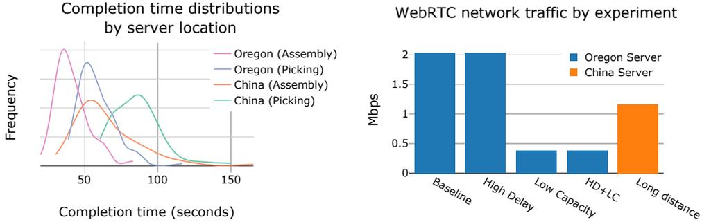
Figure 6: **System Stress Test**: Left: Comparison of completion time distributions between servers located in Oregon vs. in China, when tested from California. Right: Comparison of average throughput of video stream by network experiment, as well as for cross-pacific experiments.
