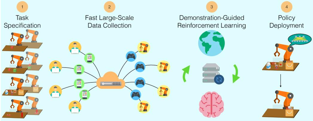
Figure 1: **System overview of ROBOTURK.** ROBOTURK enables quick imitation guided skill learning. Our system consists of the following major steps: 1) specifying a task, 2) collecting a large set of task demonstrations using ROBOTURK, 3) using demonstration-augmented reinforcement learning to learn a policy, and 4) deploying the learned skill in the domain of interest.
