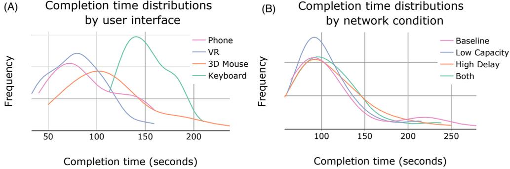
Figure 5: **System Analysis:** (A) Comparison of completion time distributions of different user interfaces on the *picking* task. (B) Comparison of completion time distributions of different network conditions using the phone interface for the *picking* task.
