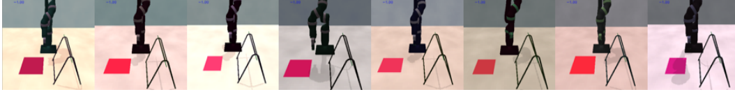
Figure 2: Examples of domain randomisation for the hanger environment. During randomisation, we vary the table textures, cloth and arm colours, light position, camera position and orientation, cloth size and position, hanger size and position, initial arm position and size of arm base.
