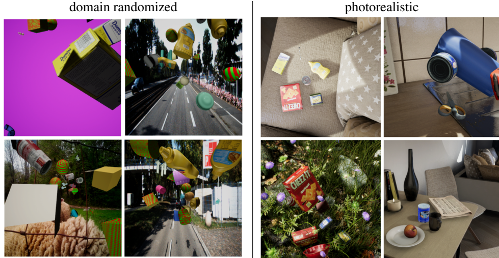
Figure 1: Example images from our domain randomized (left) and photorealistic (right) datasets used for training.
