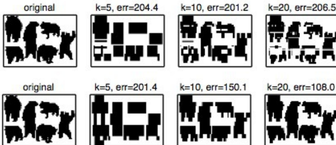
Figure 1. Example output of the baseline and our algorithm on a 700 \times 490 black-and-white image. The top row shows the output for various values of k for the baseline; the bottom row shows the output of our algorithm. The Frobenius norm error is also shown for each k .
