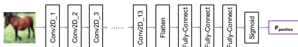
Figure 1. Network for images in CIFAR10 dataset. Each convolutional and fully-connected layer is followed by a batch normalization layer and a ReLU activation layer, which are omitted for simplicity.
