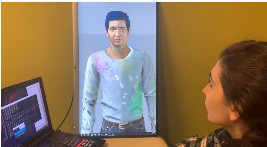
Figure 2: An example setup of the interaction with the M-Path system, where the 3D embodied conversational agent conducts Big-5 questionnaire with the participant using a webcam and microphone.
