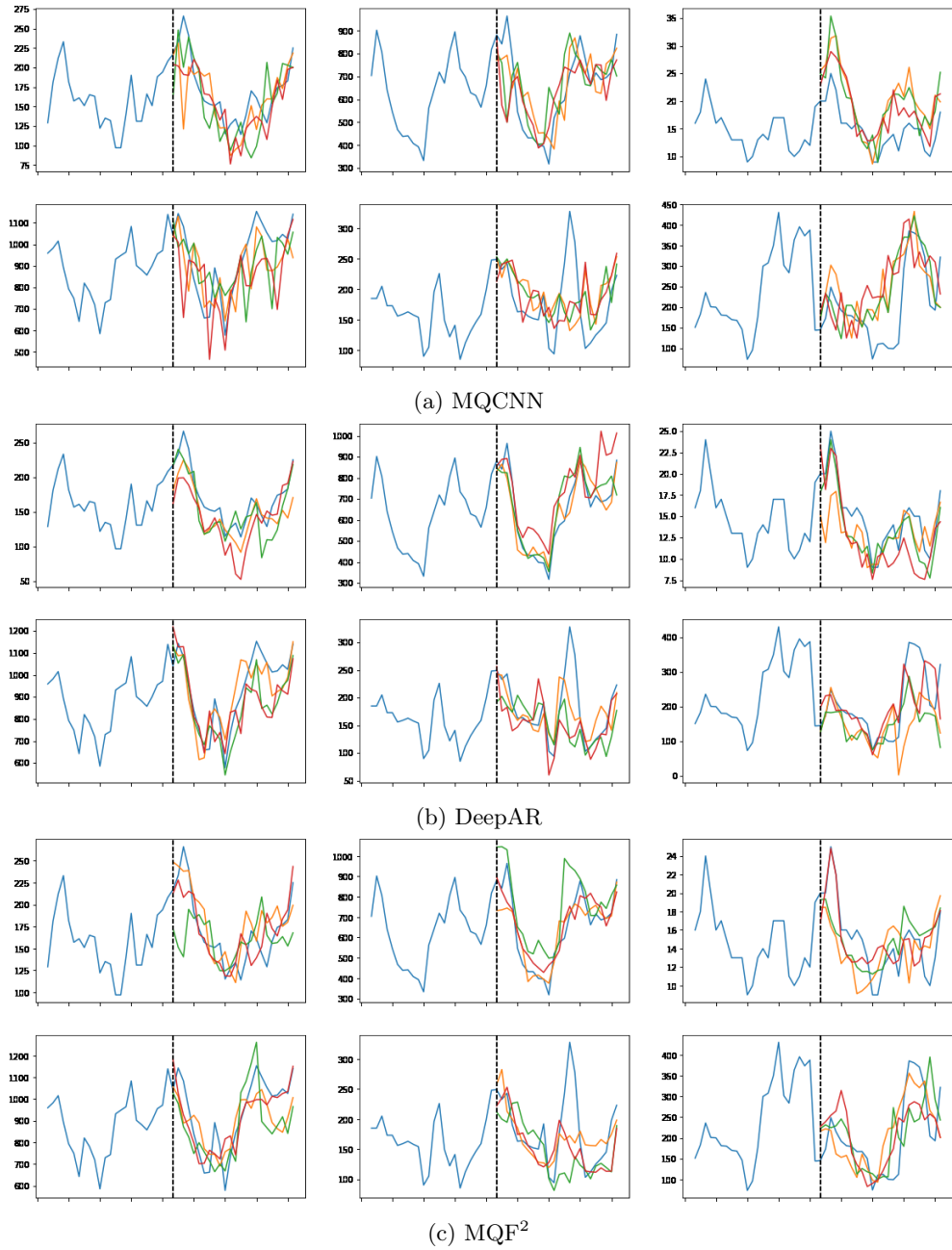
Figure 6: Sample paths generated by MQCNN, DeepAR and MQF 2 . Three sample paths are generated for each of the 6 time series of the El ec dataset. The dotted vertical lines represent the start of the prediction horizon.
