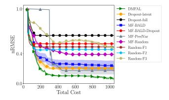
Figure 7: Normalized root-mean-square error (nRMSE) for active learning of the solution field of Poisson's equation, with three-fidelity queries. The results are averaged from five runs.
