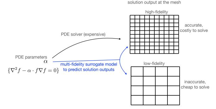
Figure 3: Illustration of the motivation and goal with physical simulation as an example. Solving every PDE from scratch is expensive. Hence, we learn a multi-fidelity surrogate model that can predict high-fidelity solution outputs outright given the PDE parameters. We develop active learning methods to further reduce the cost of running numerical solvers to generate/collect training examples.
